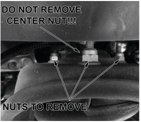
Fig. 1: Remove the three nuts. DO NOT remove the center nut.
