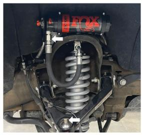
Fig. 2: Reservoir hoses facing outward (top arrow) and toward rear of vehicle (driver side view). Aluminum suspension models: loosen but do not remove nut (lower arrow).
