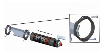
Fig. 3: Mount the reservoir to the brackets.
